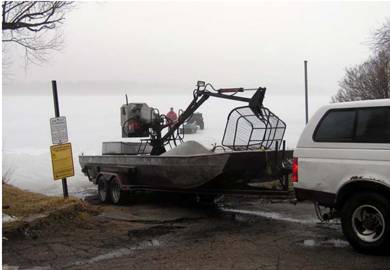
32) Warmer weather brings fog and slush on the Lake. This boat is equipped with a boom and sorting table.
