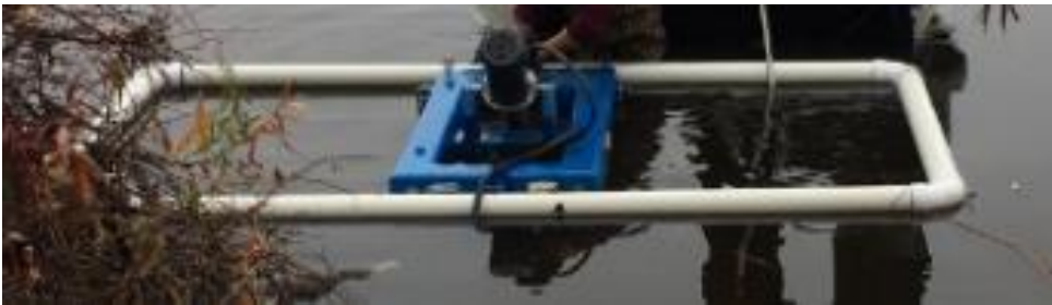
Aerator motor and float (redesigned for more support in 2017 with outrigger PVC)
