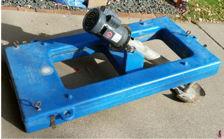
Aerator motor and float (redesigned for more support in 2017 with outrigger PVC)
